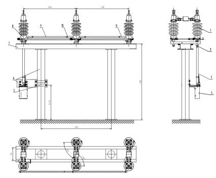
GW4-40.5 disconnector 3P linkage installation diagram
