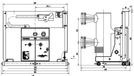
Note: The stroke of handcart is 200±2mm, and the meshing size of dynamic and static contacts is  $\geq 15 \text{mm}$ .
