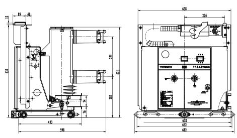
Note: The stroke of handcart is 200±2mm, and the meshing size of dynamic and static contacts is  $\geq 15$ mm.
